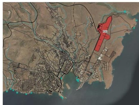
Map Legend Airport Administrative boundary Roads Flood hazard Coastal flooding area including sea-level rise by 2100 (+0,7m) and high tidal coefficient (113) Waterways Potential flooding area 0 0.5 1 km RESALLIENCE VIGNOTE (2019) Sources : VINCI Airports (2019) ; CGAR CSI (2019) ; OpenStreetMap (2019) ; Bing Satellite (2019) ;
